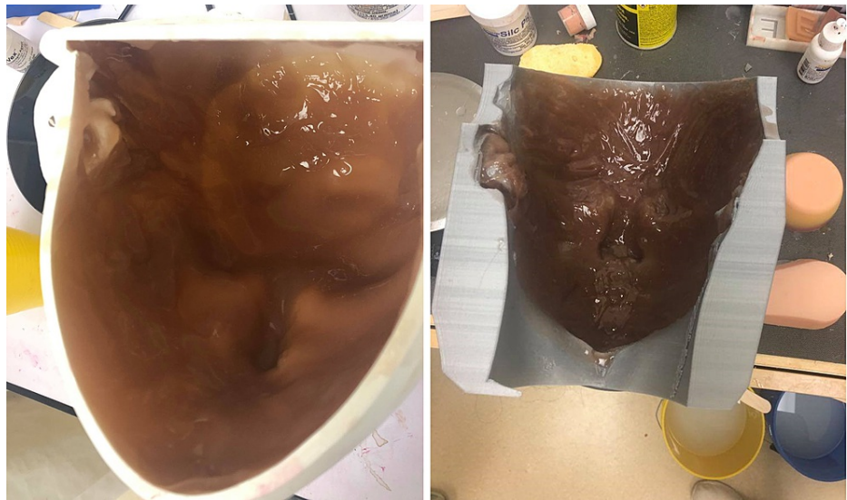
FIGURE 4: The silicone after being poured in the molds for the Indian overlay (left) and Jamaican overlay (right).
