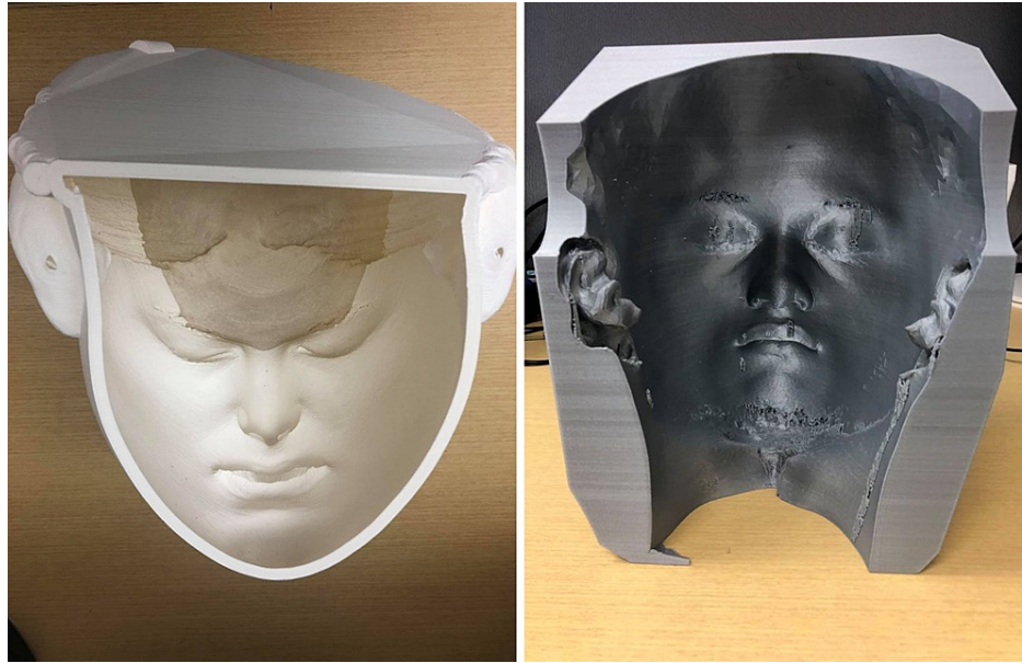
FIGURE 3: 3D printed mold of Indian scan on left, and of Jamaican scan on right.
