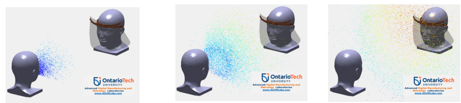
FIGURE 1: Computational Dynamics Modelling of COVID-19 Transmission From Infected Patient to Personal Protective Equipment (PPE) User via Air at 10 ms, 20 ms and 50 ms (Left to Right) Following a Sneezing Event.
