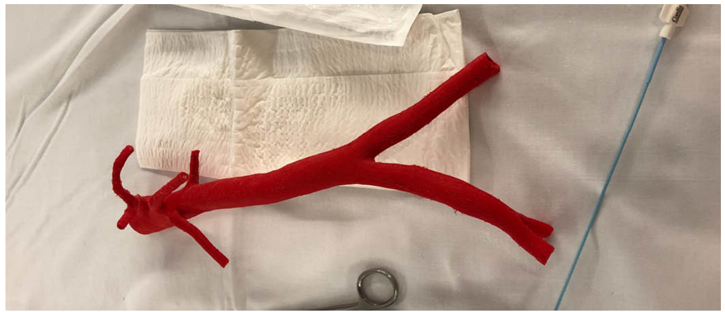
FIGURE 8: 3D-printed abdominal aorta using TPE 80A filament
