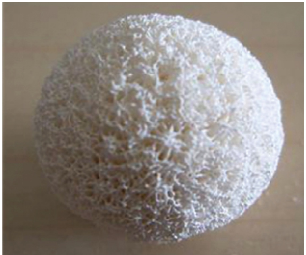
FIGURE 4: Porous Hydroxyapatite (HA) implant.
