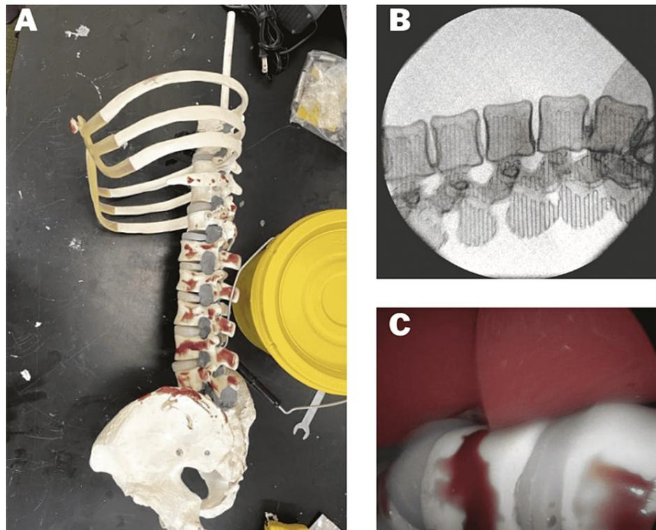
**FIGURE 3: (A) Assembled spinal module consisting of PVC pelvis and sacrum, 3D-printed ABS L1-L5, silicone discs, and PVC T8-T12 vertebrae with partial rib cage. (B) Lateral fluoroscopic imaging of a 3D-printed ABS L1-L5 model including the iliac crest. (C) Laparoscopic image of synthetic psoas muscle atop of L2-L3 3D-printed vertebrae with silicone intervertebral discs.**
