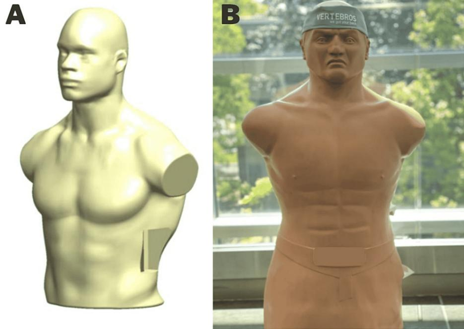
**FIGURE 1: (A) Computer-aided design rendering of synthetic silicone and polymer foam torso housing. (B) Silicone and polymer foam torso shell were used in the construction of the lateral access training model.**
