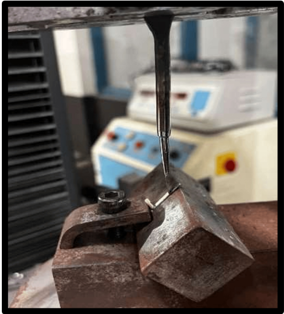
FIGURE 4: Fractured specimen obtained after the application of load
