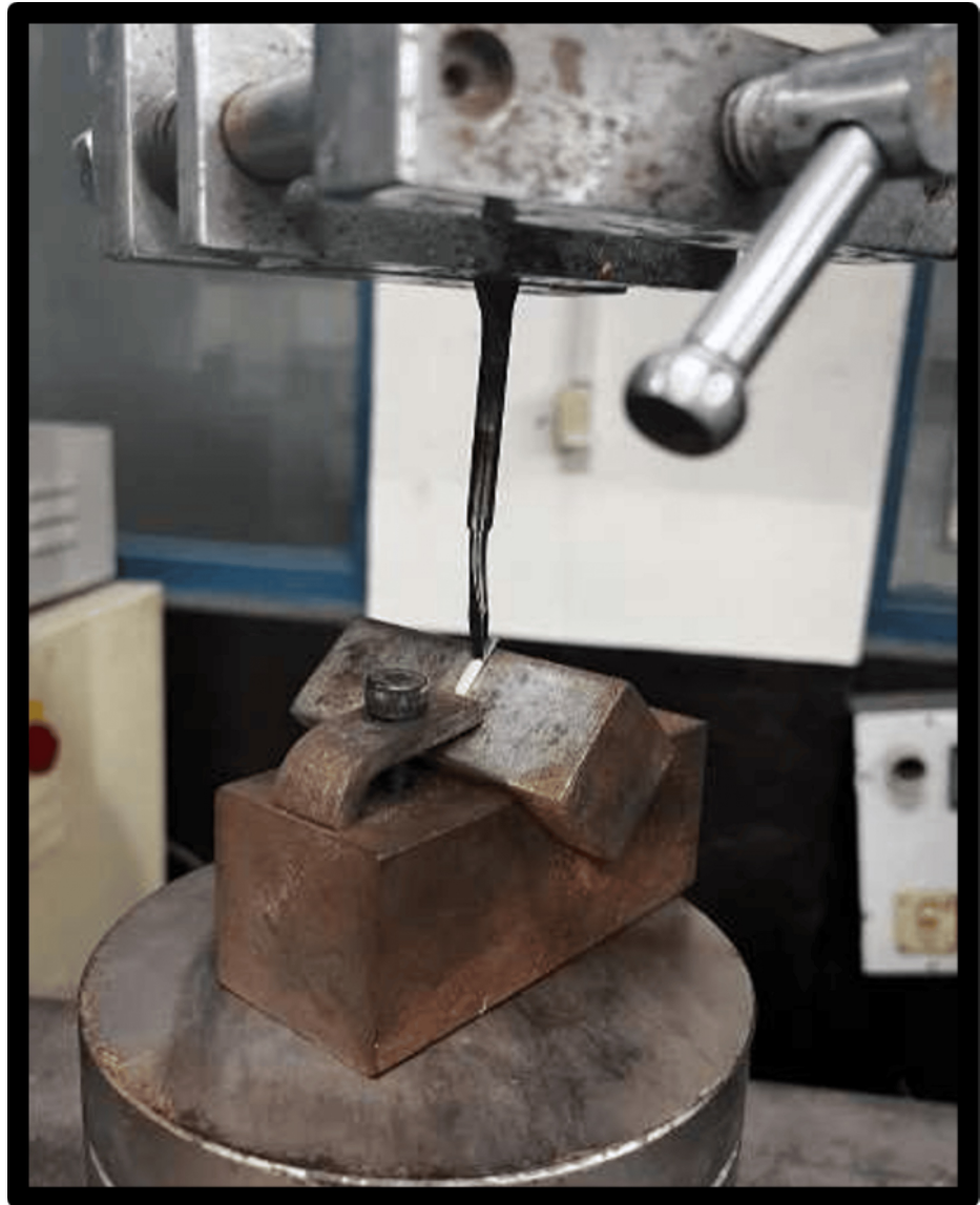
FIGURE 3: Testing for shear bond strength on the universal testing machine
