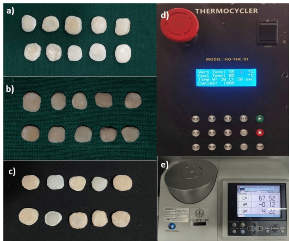
FIGURE 3: Colour change observed in the individual groups following thermocycling.
