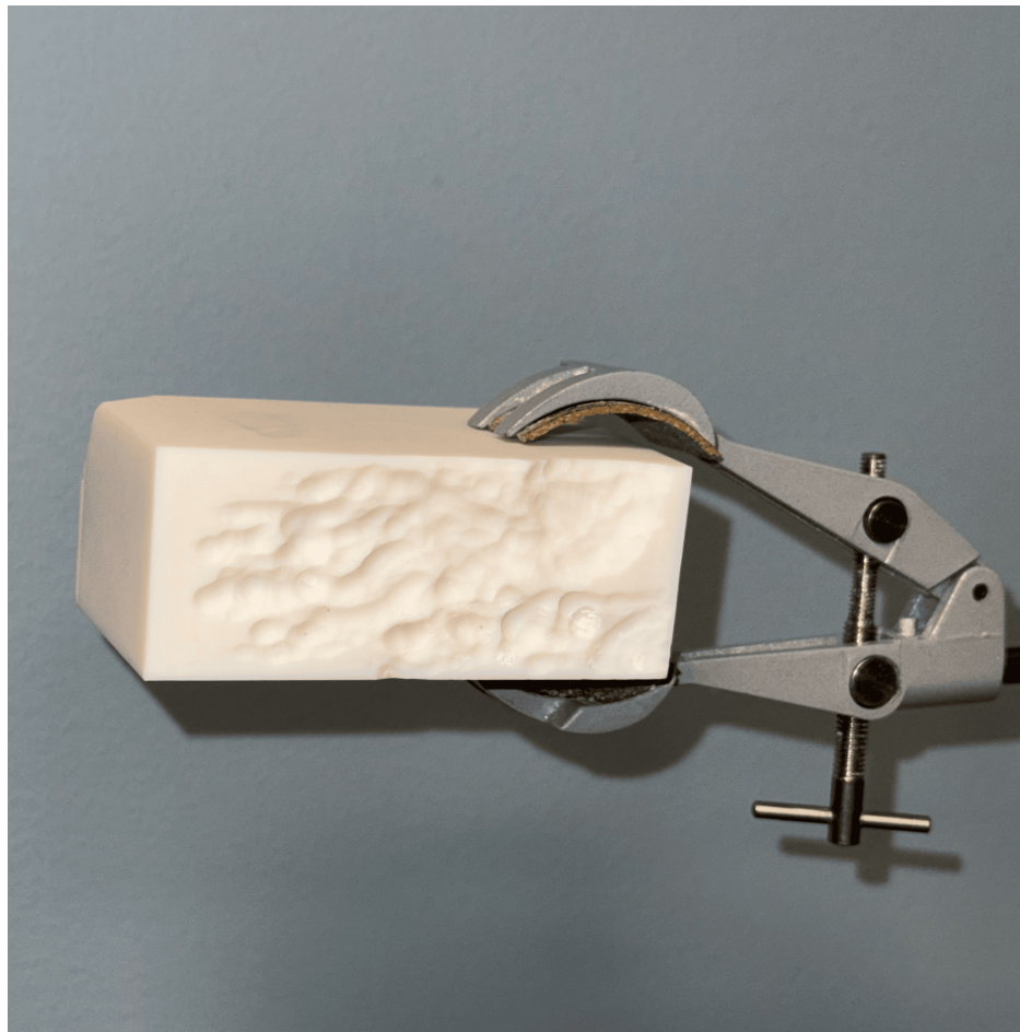
FIGURE 1: Cortical bony configuration of the AMTB analog
