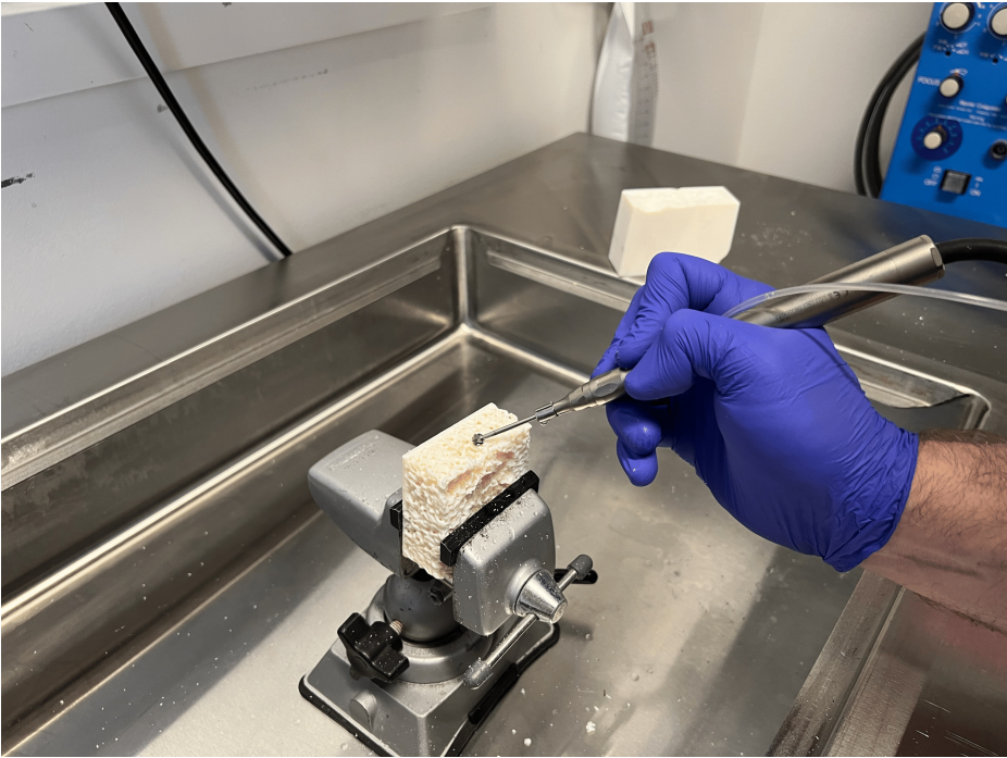
FIGURE 3: Laboratory setup for drilling the AMTB analog
