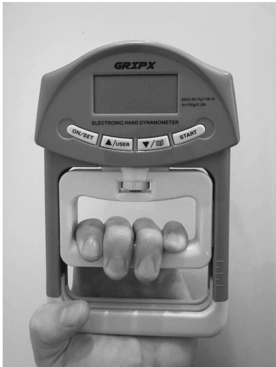
FIGURE 1: Dynamometer used in the measurement of the grip strength.
