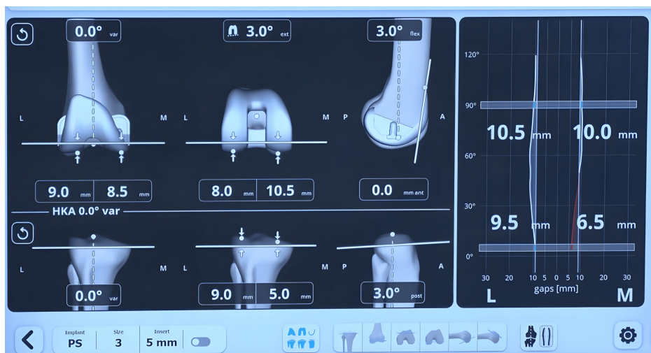
FIGURE 3: Manufacturer's software showing the femur implant size and default femur component flexion and external rotation
