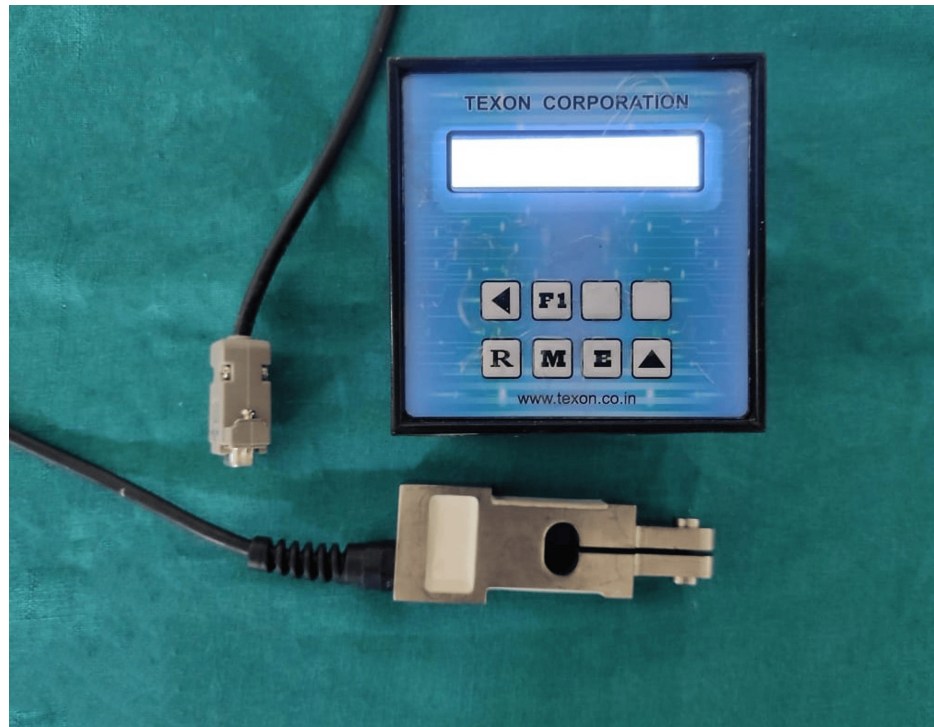
FIGURE 3: MBF was measured using a gnathodynamometer (Texon Co. Ltd., Uijeongbu-si, Republic of Korea).
