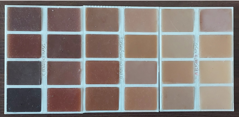
FIGURE 2: 3D printed shade guide consisting of 24 shades, eight subshades of light (L), eight subshades of medium (M), and eight subshades of dark (D). Source: Original work by the author.
