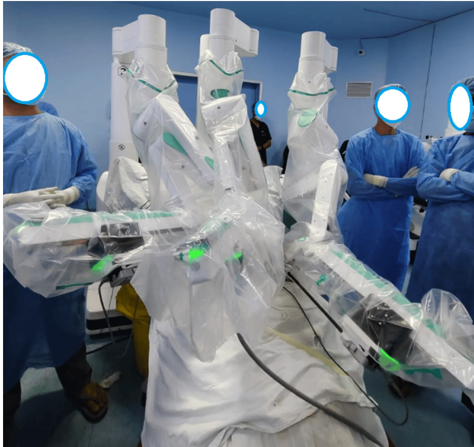
FIGURE 5: Docked patient side arm cart with robotic arms
