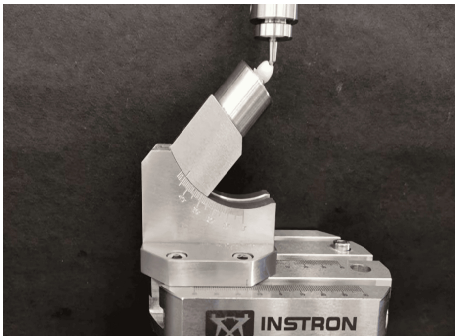
FIGURE 6: Fracture loading of ZLS post & core in a Universal Testing Machine.
