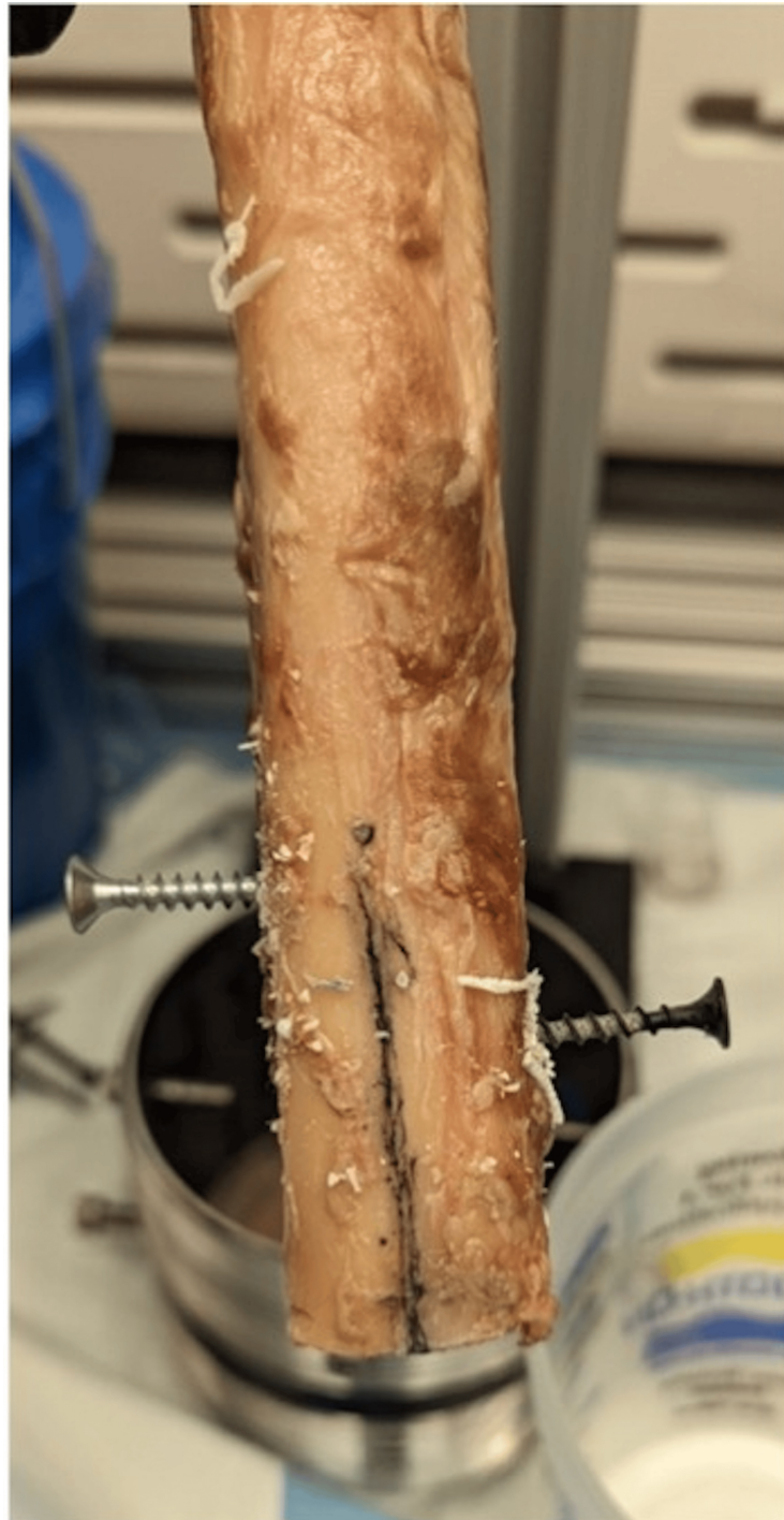
FIGURE 3: Structural screws driven into the distal aspect of the implanted specimen to improve mechanical locking of the bone into the potting resin
