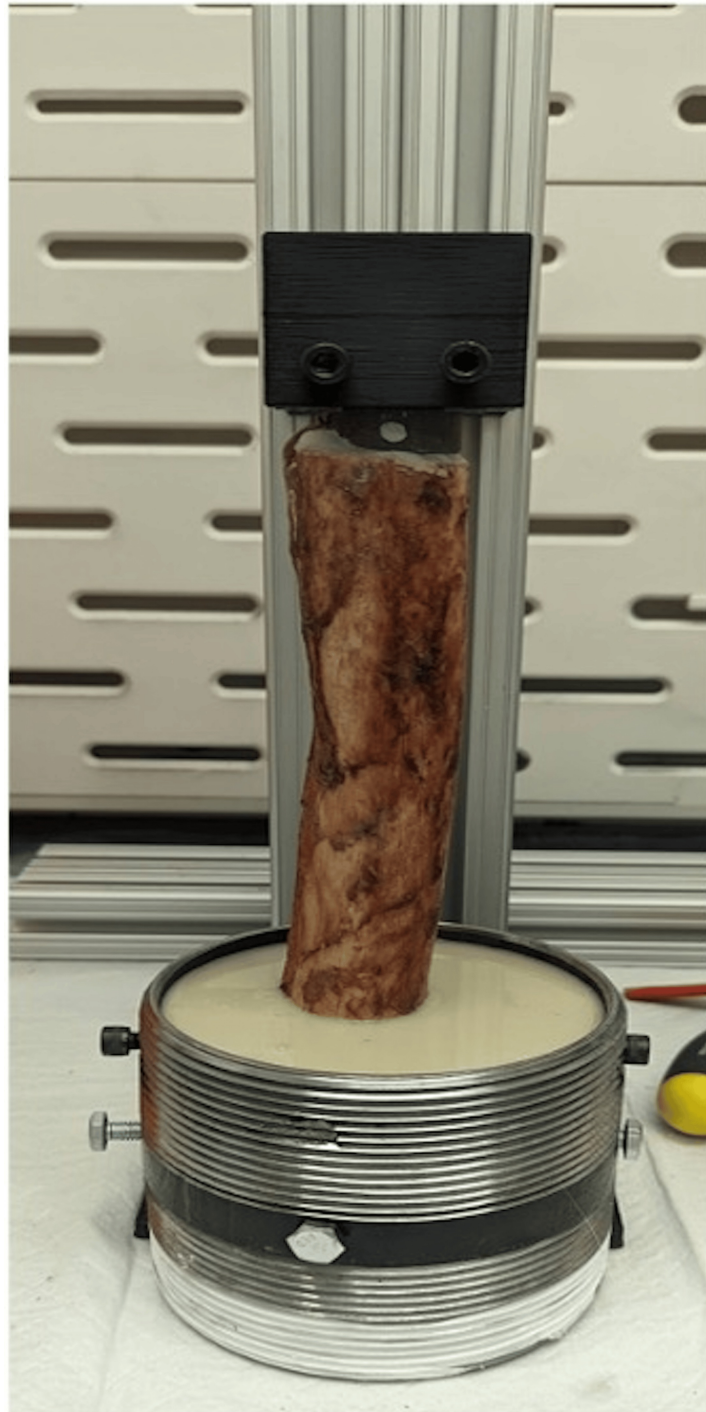
FIGURE 5: Final potting construct after resin curing for at least 60 minutes
