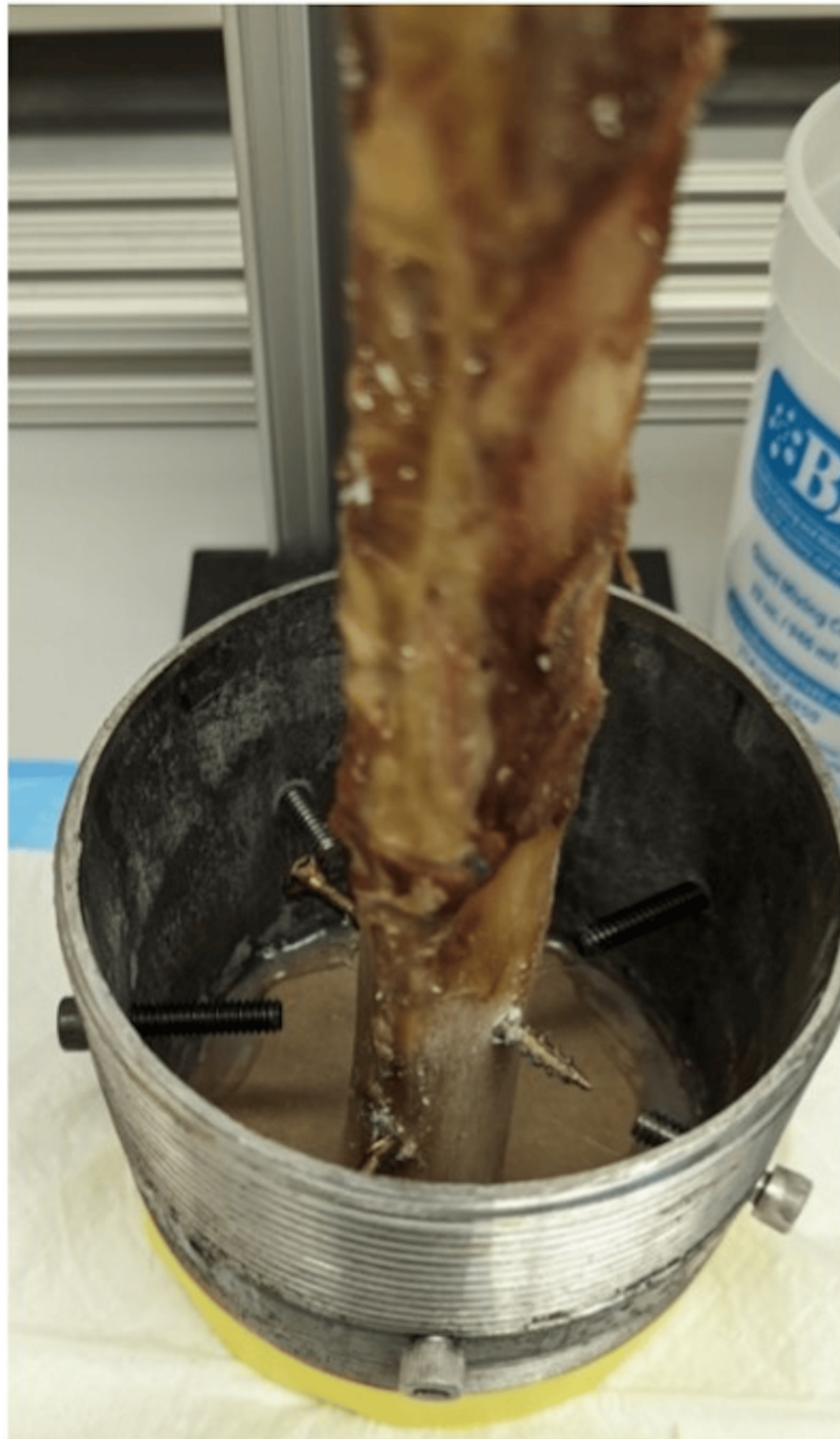
FIGURE 4: Implanted specimen in a 4-inch iron pipe fitting in preparation for urethane casting resin
