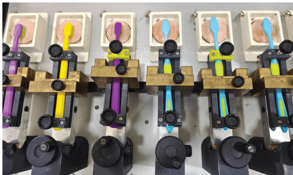
FIGURE 6: Apparatus used for brushing simulation (SD MECHATRONIK Toothbrush Simulator ZM-3.8)
