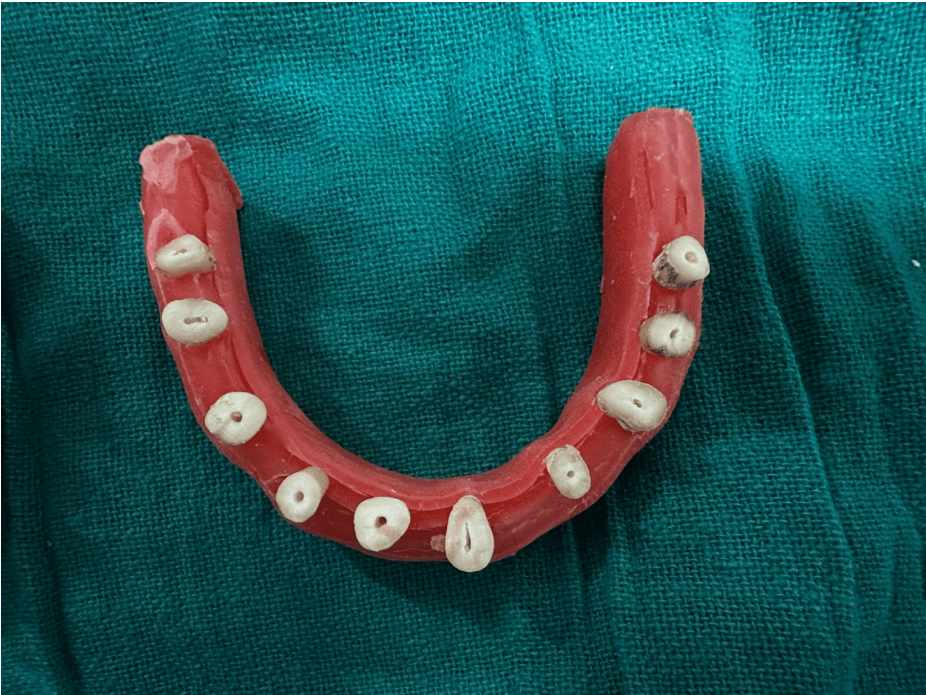
FIGURE 1: Sample mounting on modeling wax
