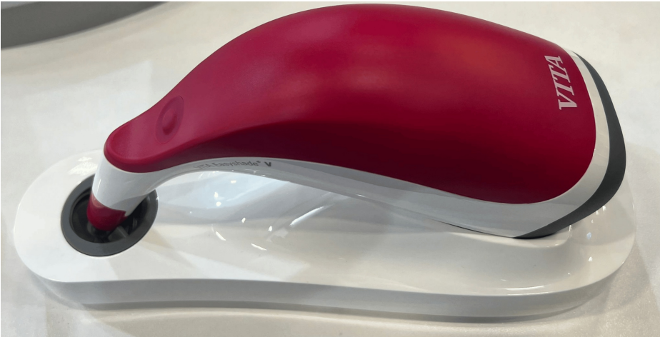
FIGURE 2: Vita Easyshade V Spectrophotometer used for colour measurement in the study
