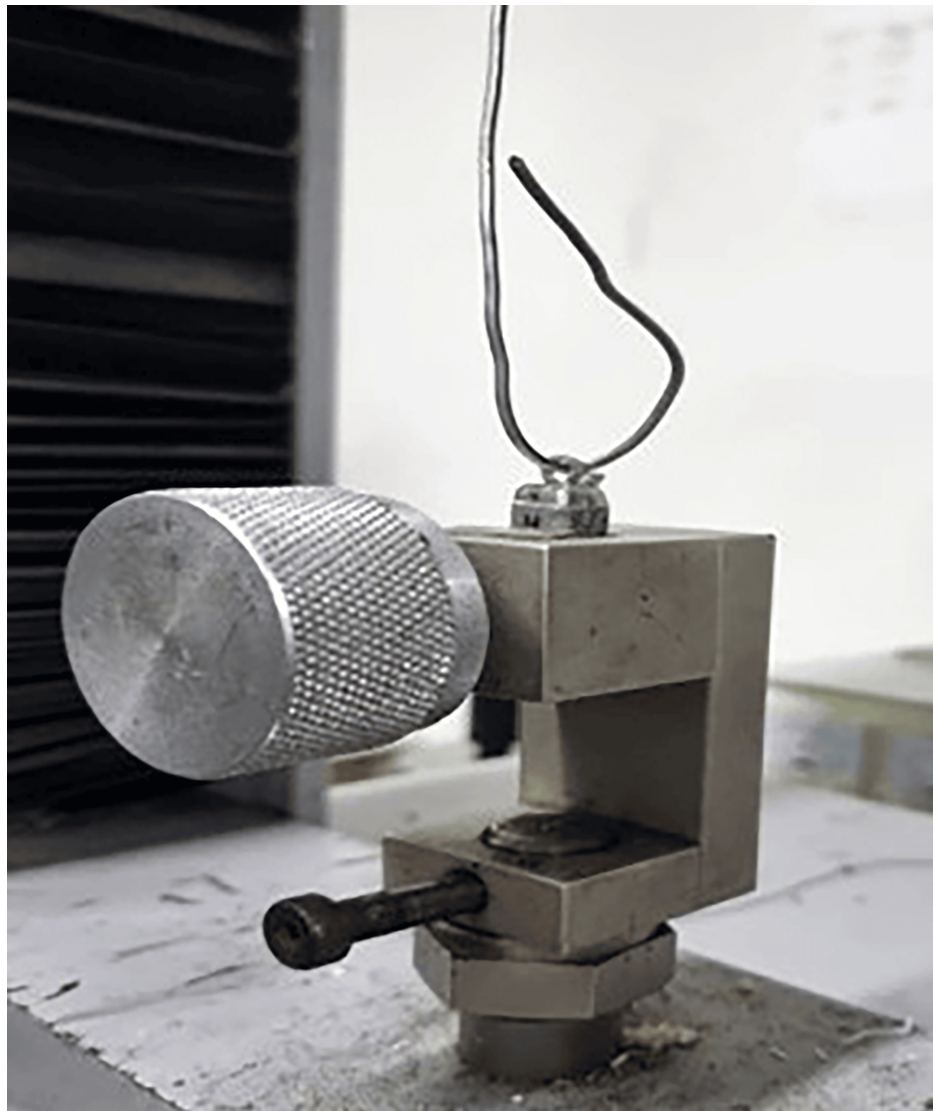
FIGURE 6: An abutment in the testing machine.
