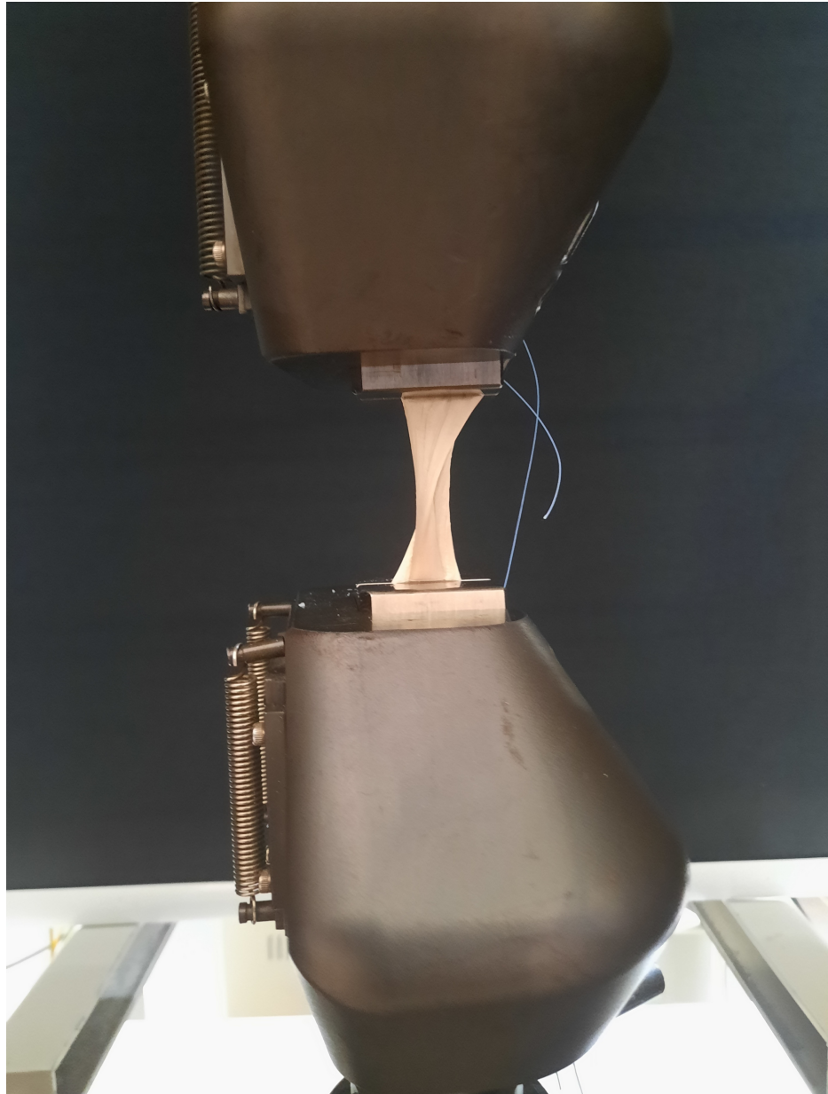
FIGURE 3: Measuring the tensile strength of tendons using the Shimadzu Autograph AG-IS 100 kN device.
