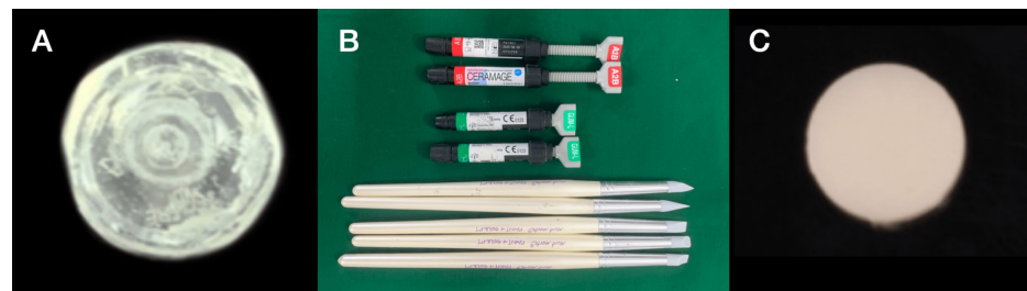
FIGURE 2: Silicone mould fabrication followed by indirect composite disc preparation after polishing.
