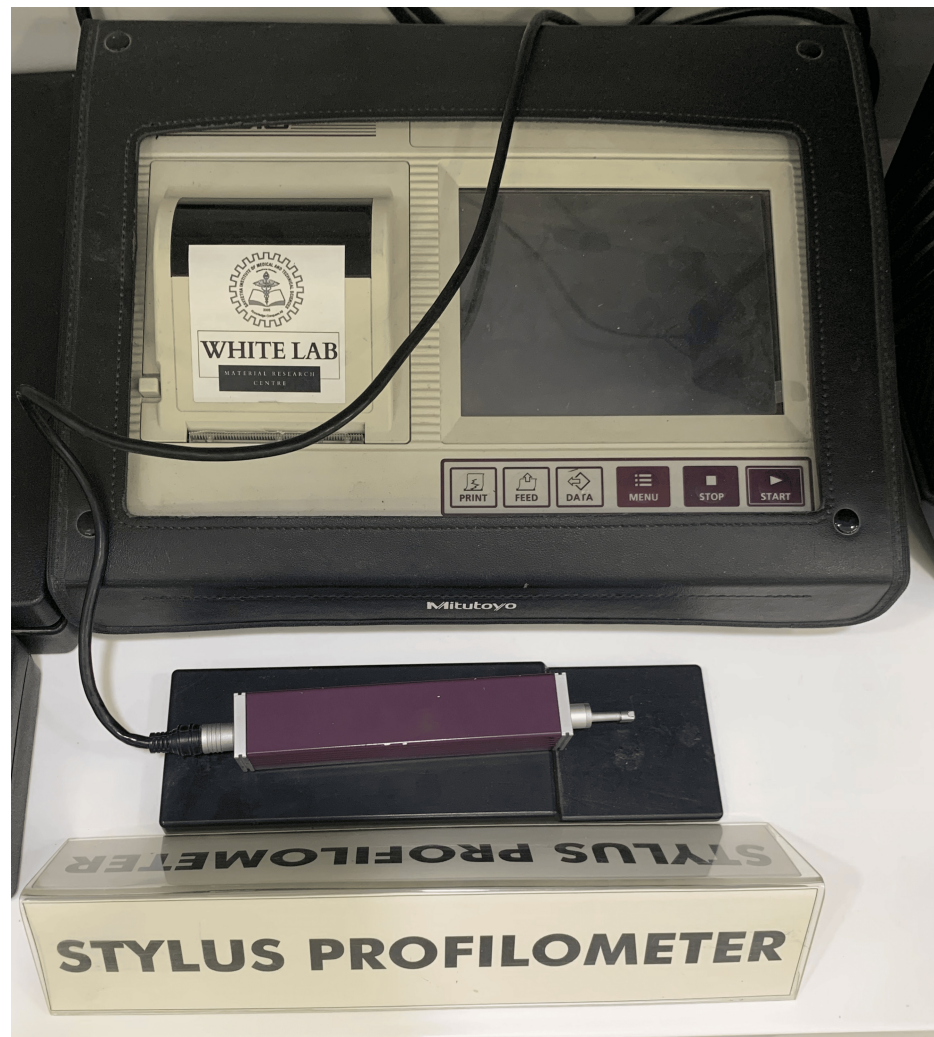
FIGURE 5: Stylus profilometer used to test the surface roughness.
