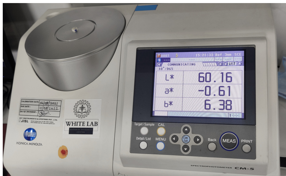
FIGURE 4: Evaluation of color using a spectrophotometer
