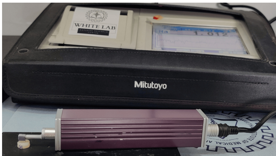
FIGURE 2: Evaluation of surface roughness using surface profilometer
