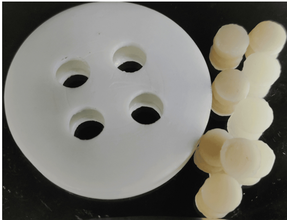
FIGURE 1: Teflon mold and composite resin samples
