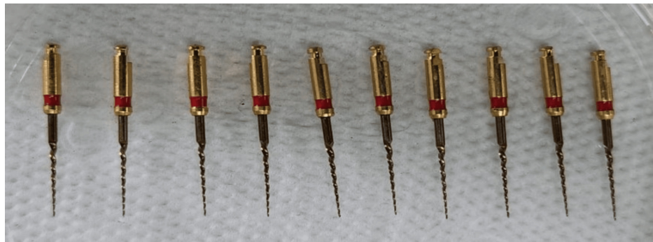
FIGURE 2: Endodontic files after the titanium oxide coating removal procedure
