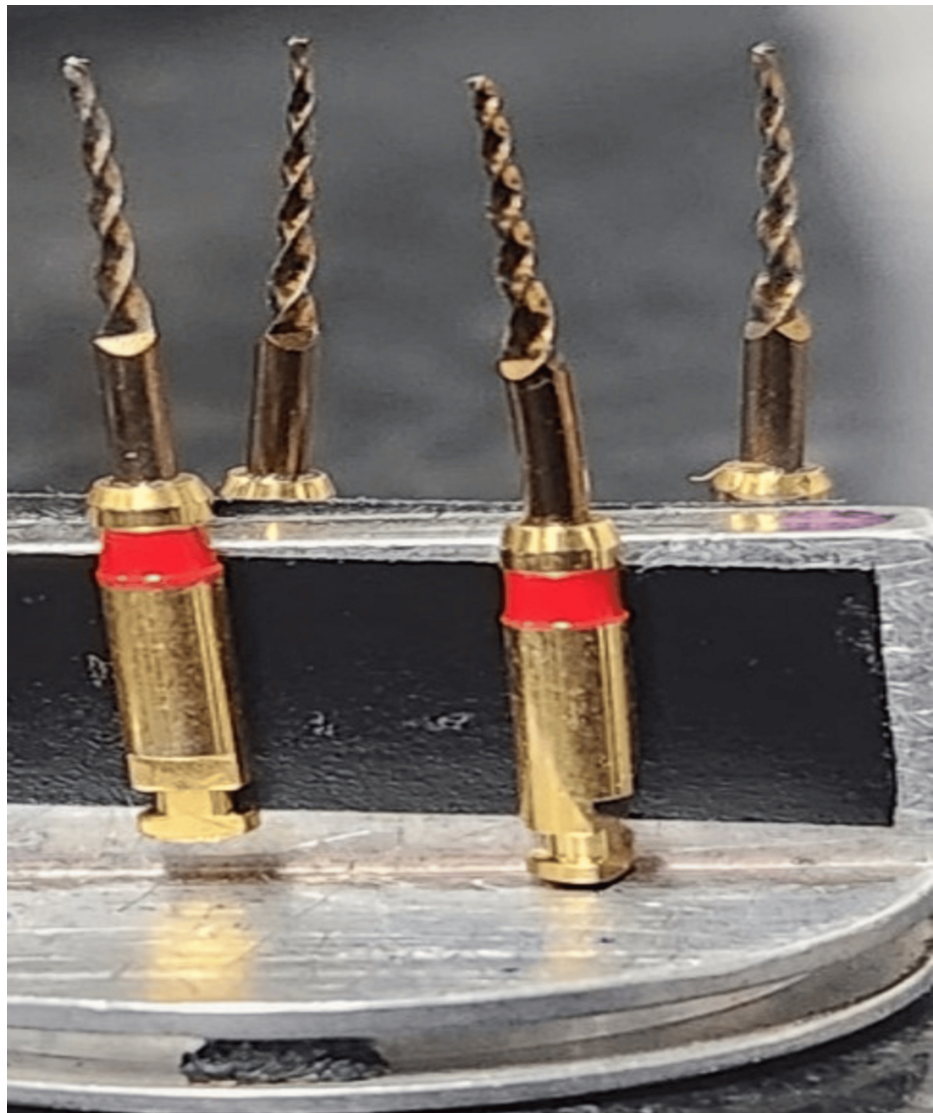
FIGURE 4: Endodontic files mounted on metallic stubs for SEM analysis
