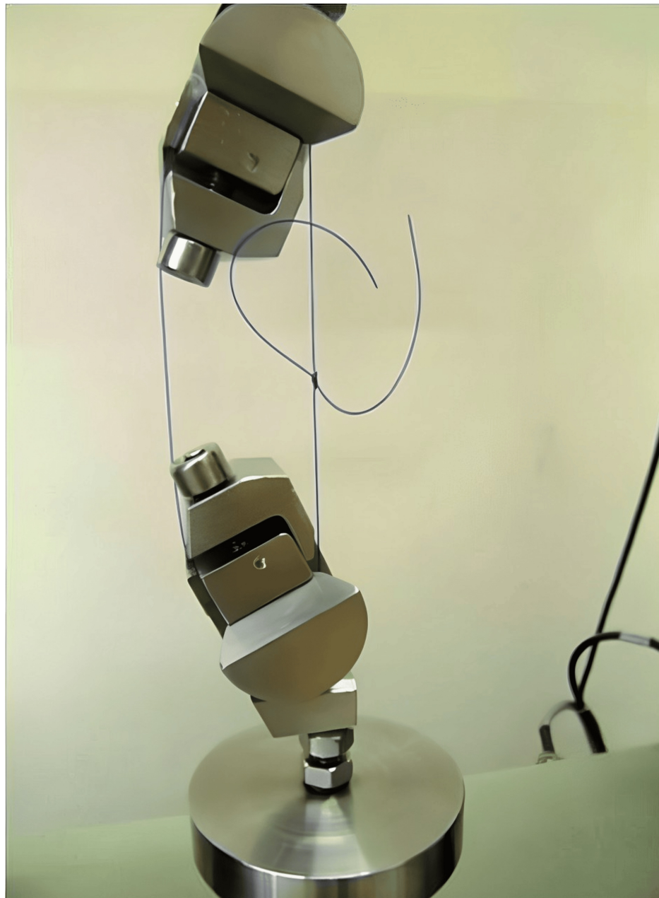
FIGURE 1: Universal testing machine for the suture thread
