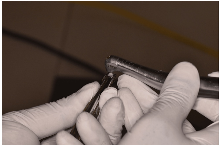
FIGURE 1: Laser treatment on bracket bases using Waterlase iPlus laser system
