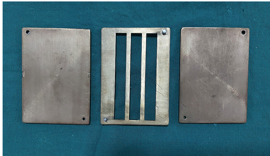
FIGURE 1: Custom fabricated brass die of 12 x 6 cm with three slots of 80 x 10 x 4 mm
