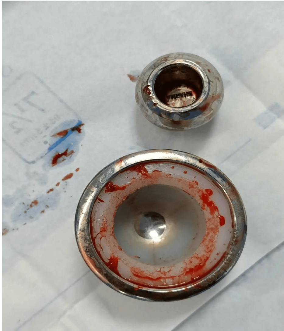
FIGURE 3: Retrieved bipolar head assembly after removal, showing complete wear-through of the polyethylene liner within the cup with a resulting metal-on-metal articulation between the inner and outer heads.
