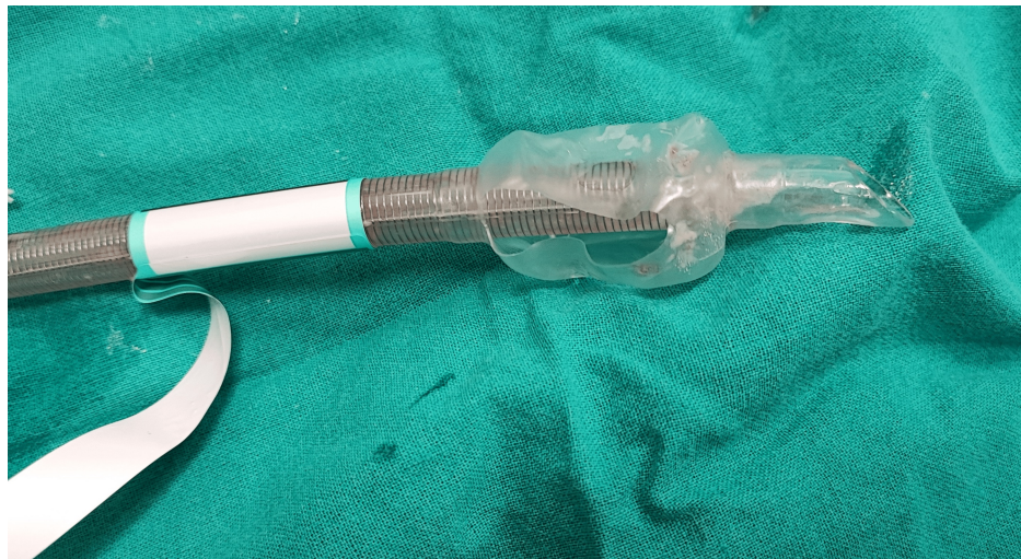
FIGURE 2: Postextubation view of the electromyographic endotracheal tube showing the focal cuff defect.
