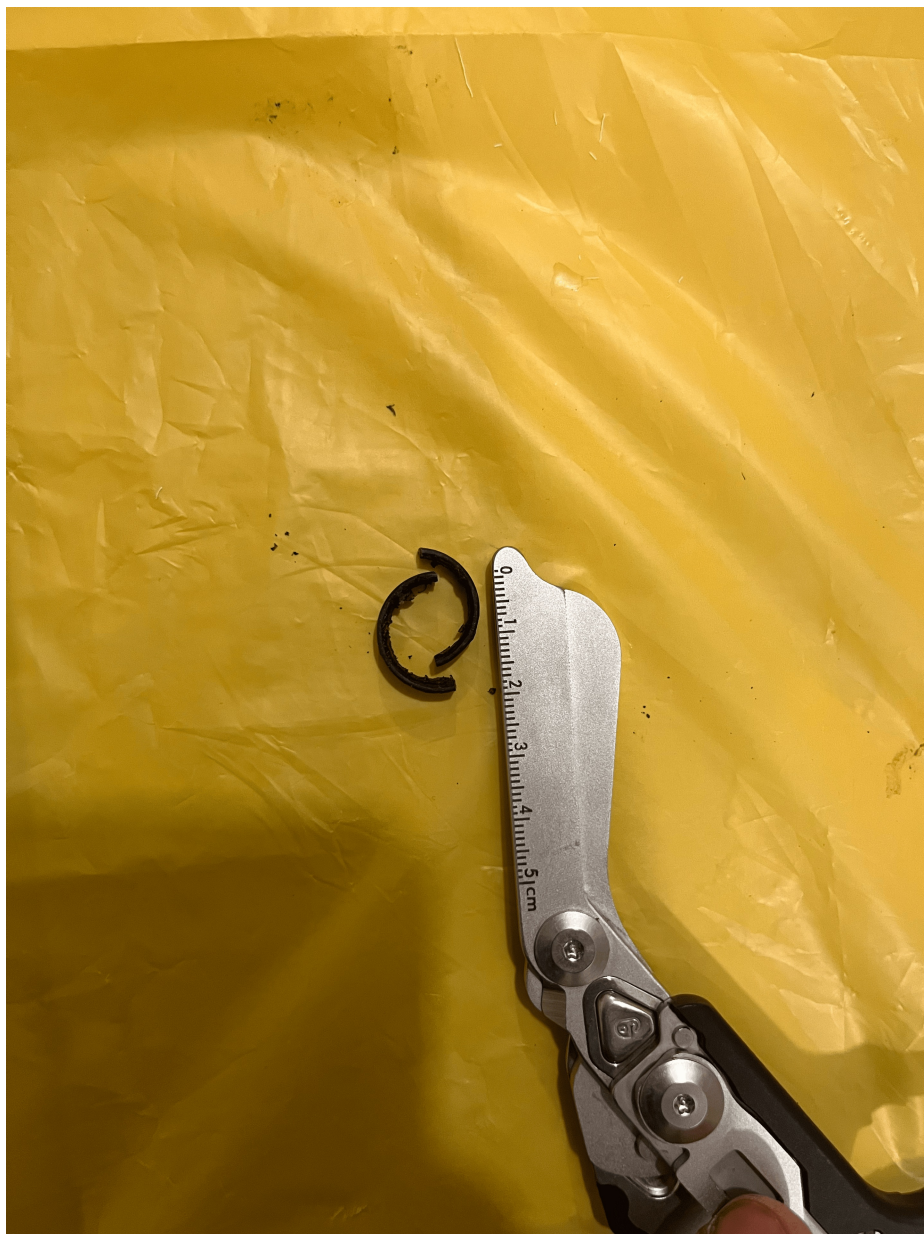
FIGURE 8: Showing ring cut in two places for easy removal
