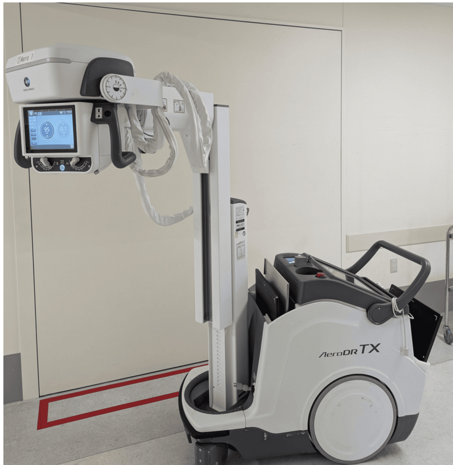
FIGURE 5: Photograph of the mobile dynamic digital radiography equipment (AeroDR Trauma & X-ray; Konica Minolta, Chiyoda City, Japan), which has a portable detector panel.
