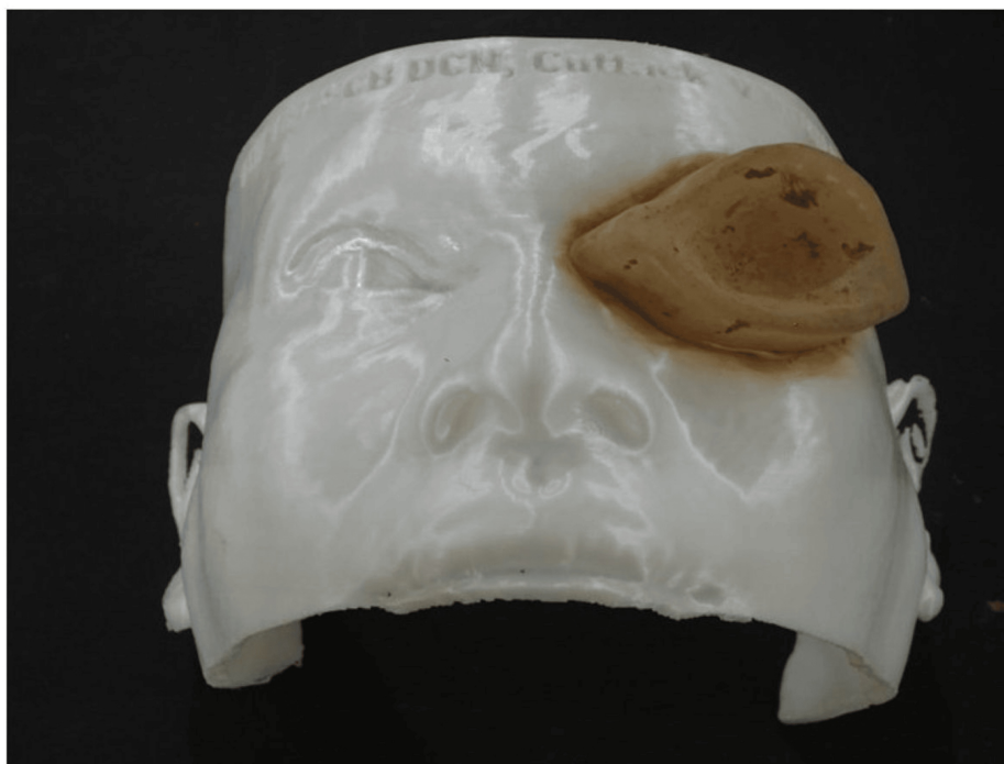
FIGURE 4: 3D-printed resin mold used for fabricating the silicone prosthesis.
