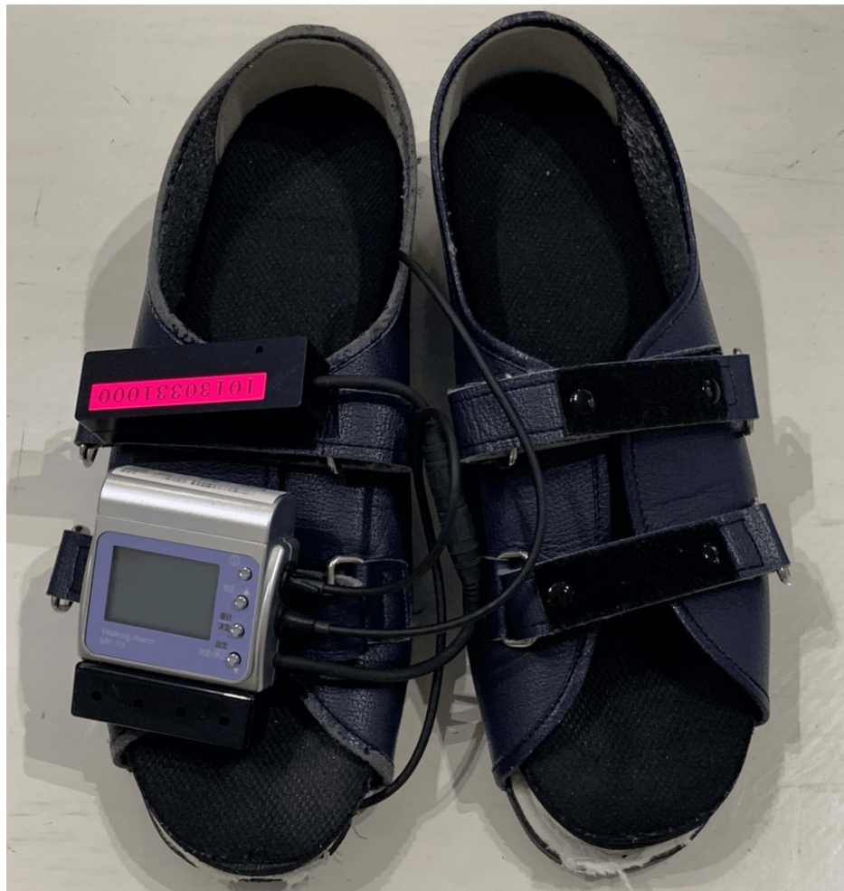
FIGURE 3: Shoe-based lower-limb load meter.
