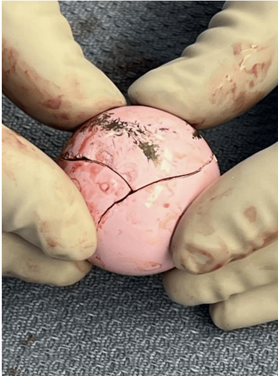
FIGURE 3: Proximal side of the fractured ceramic head components pieced together following removal.
