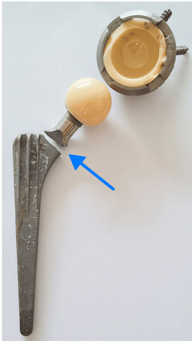
FIGURE 2: Postoperative picture of the broken femoral stem
