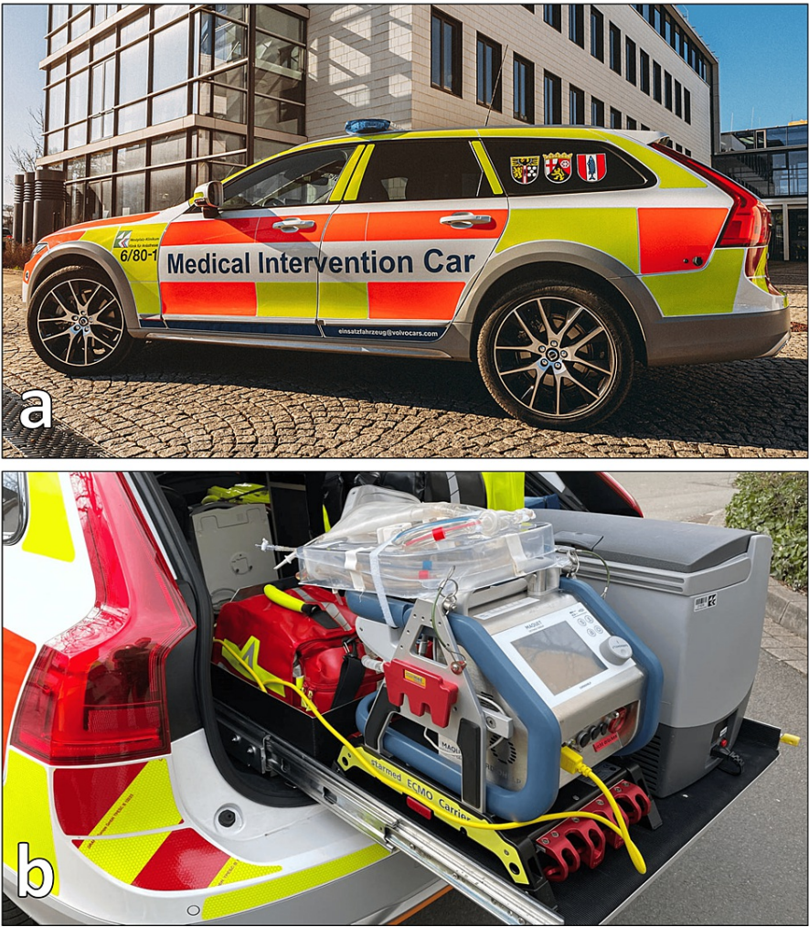
FIGURE 1: a. The medical intervention car (MIC) utilized within our hospital. b. The extracorporeal life support (ECLS) device which is transported in the MIC.
